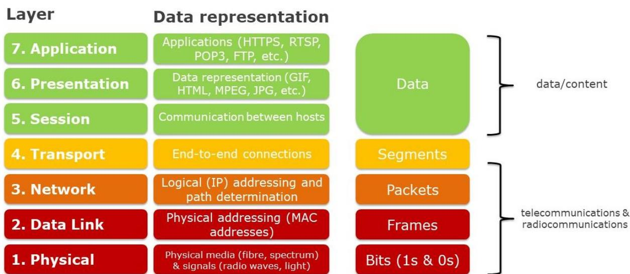
Figure 1: The Open Systems Interconnection (OSI) model
